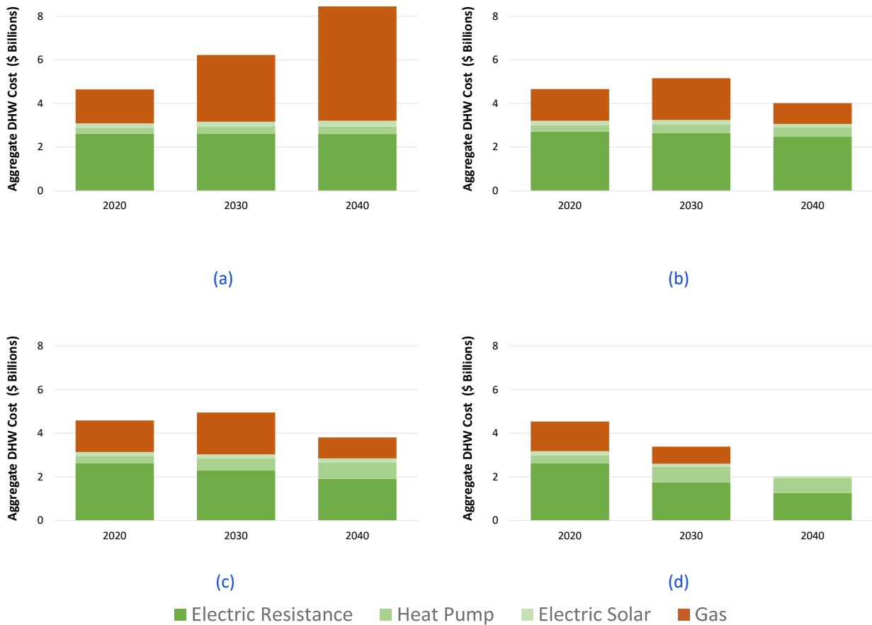
Figure 15. Aggregate DHW operating costs across the NEM. (a) Business as Usual. (b) Highly Flexible. (c) Highly Efficient. (d) Rapid Electrification.
