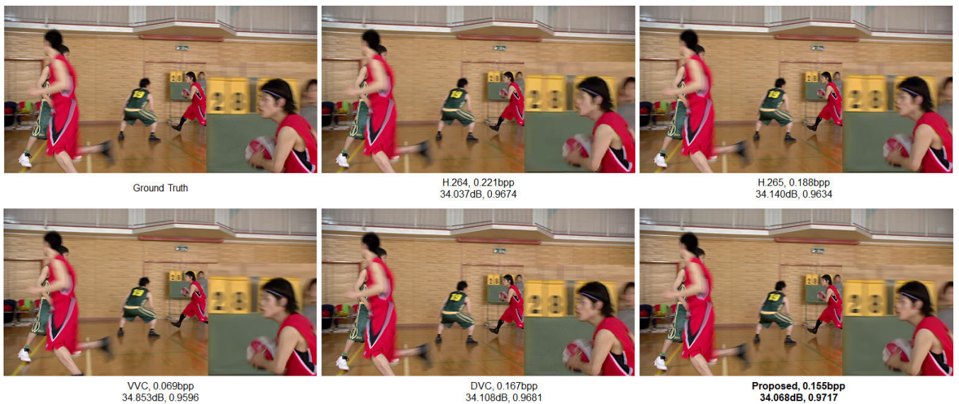
FIGURE 9. Visual quality comparison of the reconstructed frame from VVC Class B dataset.
