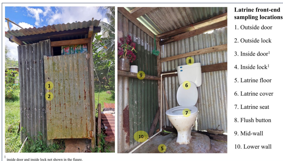
Fig. 2 In-depth front-end sampling locations of a cistern-flush latrine at Natadradave, Dawasamu, catchment. The yellow circles with numbers represent the sampling locations
