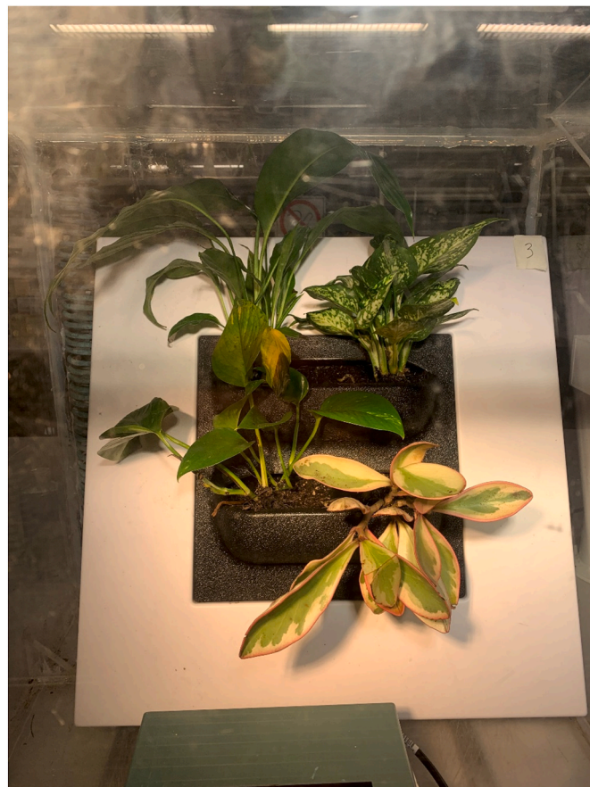
Fig. 1. Experimental small-scale green wall biofilters maintained within climate-controlled research glasshouse. (For interpretation of the references to colour in this figure legend, the reader is referred to the Web version of this article.)
