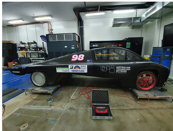
Figure 1. Measurement setup to determine the center of gravity.
