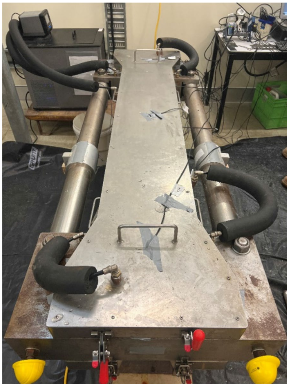
Fig. 3 Test of rigid cracking frame
