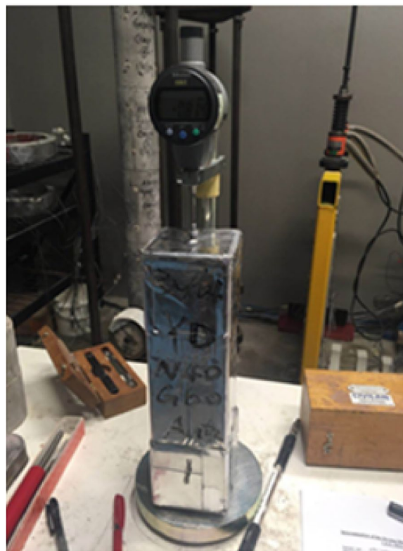
Fig. 5 Autogenous shrinkage specimens
