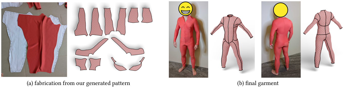
Fig. 26. A fabricated wetsuit. The input 3D garment model is based on a 3D scan of the subject. The open collar will be replaced with a zipper in the final garment. It took around 5 hours for a single person to prepare the pieces, cut, and sew.
