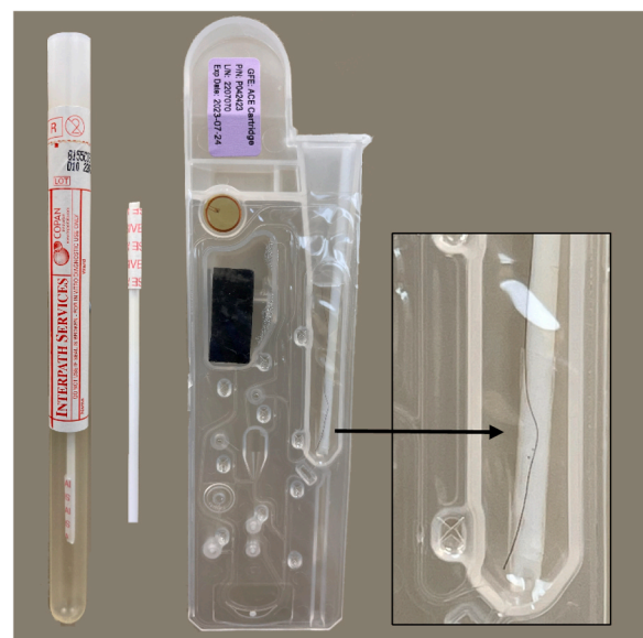
Fig. 1. Modified swab for hair samples using a rayon swab and ~2 mm x 19 mm of double-sided tape and the RHID ACE GFE cartridge with a hair sample inserted.
