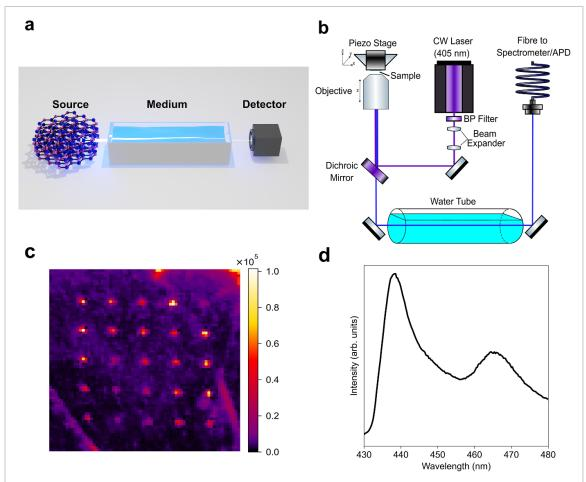
**Figure 1.** (a) 3D representation of a B-centre in hBN propagating through water. (b) Simplified schematic of the confocal setup used in this work, incorporating a 1 m tube of water in the collection path. All components are labelled in the figure. Excitation is performed using a 405 nm laser through a high numerical aperture objective. (c) A photoluminescence (PL) confocal map of a B-Centre array, engineered in a hBN flake. (d) PL spectra of a B-centre ensemble.
