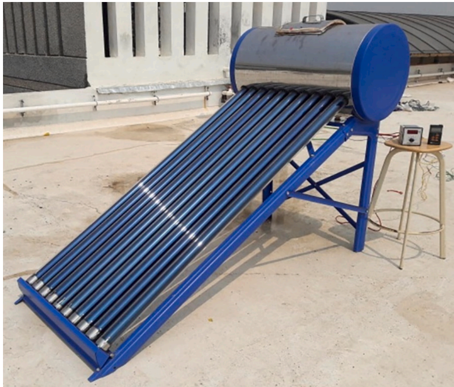
Fig. 52. The photograph solar water heater using encapsulated hybrid nano-enhanced PCM [246].
