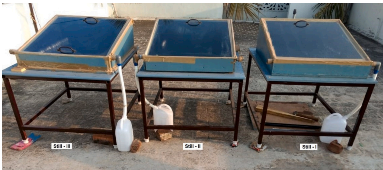
Fig. 18. Single-slope solar still by concentric tube ring encapsulated PCM [77].
