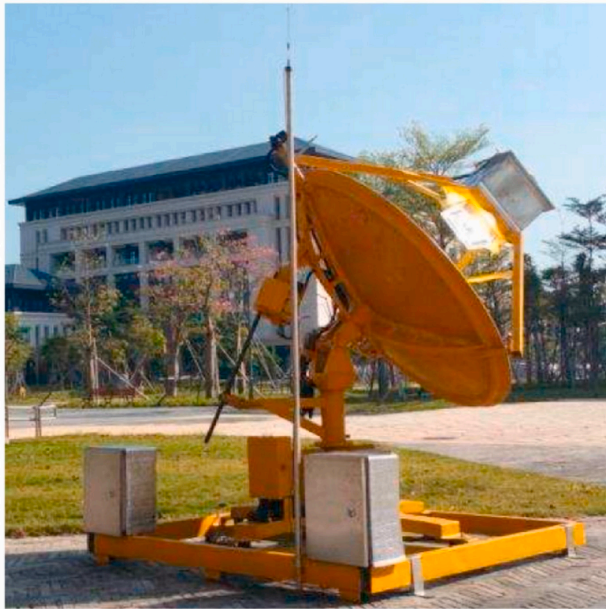
Fig. 24. Photovoltaic/thermal using solar tracking and encapsulated PCM [183].
