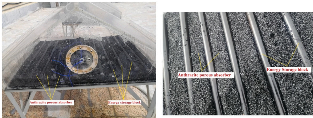
Fig. 49. Double slope solar still using encapsulated nano-enhanced PCM, nano-coated and absorber media [136].
