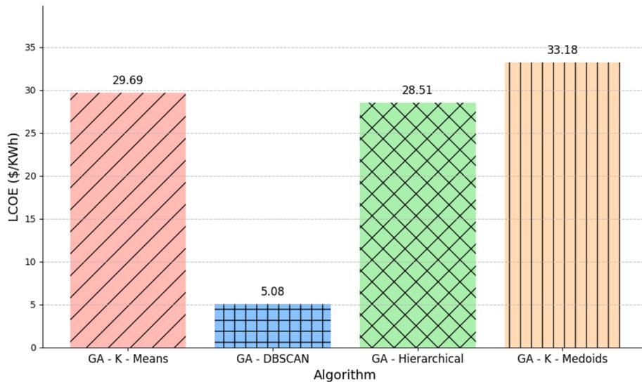
Fig. 21. Levelized Cost of Energy Comparison for these four algorithms.
