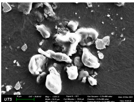
Figure 5.7. Images of Ceridust 3615 ® aggregates and micro-sized Ceridust 3615 ® model particles collected with a 0.8 μm filter. The particles were imaged using a FEG-SEM at magnifications of (A) 100 X, (B) 400 X, (C) 700 X and (D) 1500 X. Size bars of 100 μm in image A and 10 μm for images B – D.
