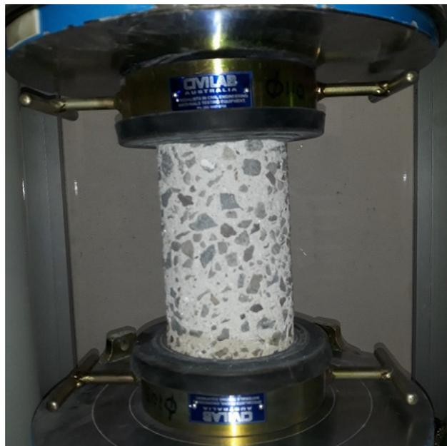
Figure 6. Rubber caps on the ends of a sample in compression test
