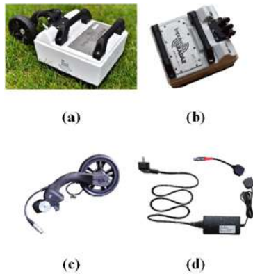
Figure 3: The GPR system. (a). The whole GPR system (b). The control unit. (c). The measurement wheel. (d). The battery
