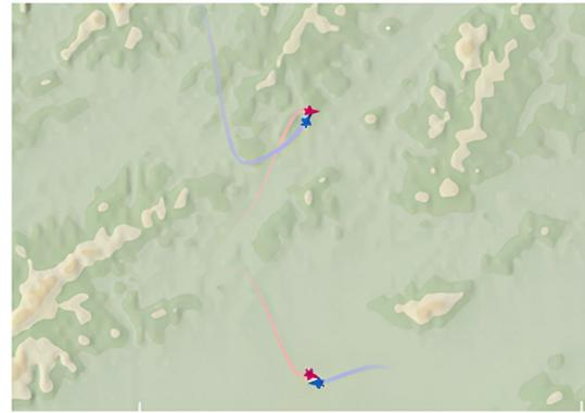
**Fig. 21** Trajectory diagram of UAVs for two-to-two pursuit and escape mission
