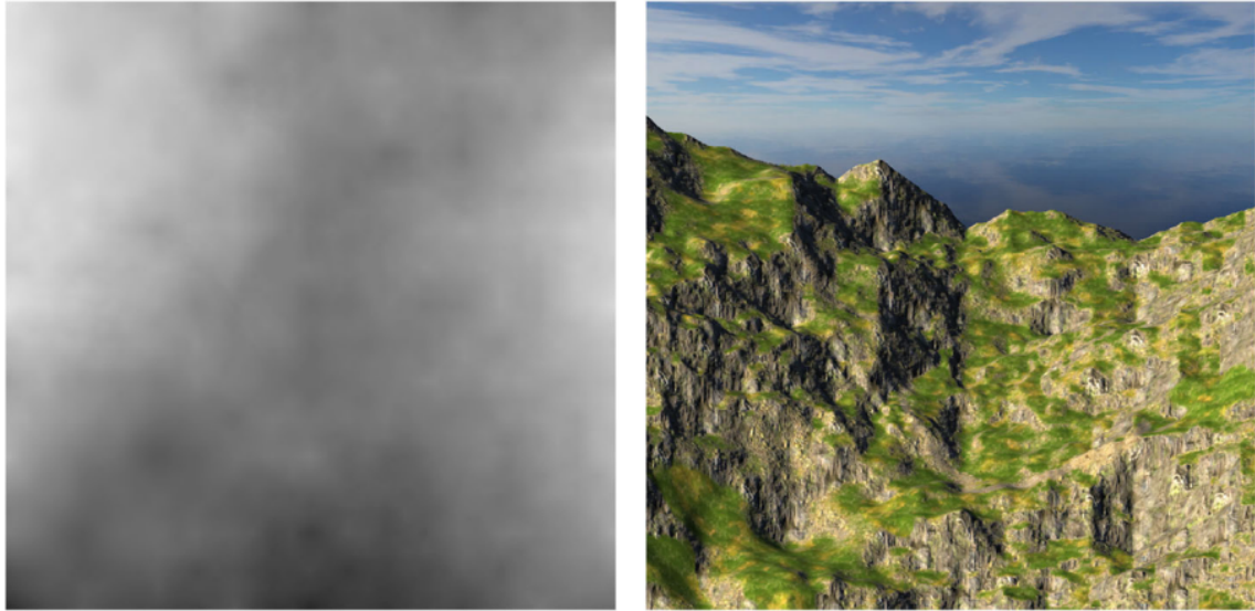
Figure 2.3: Procedural texture obtained with the Perlin method and its terrain representation (Gasch et al., 2020, Figure 2)
