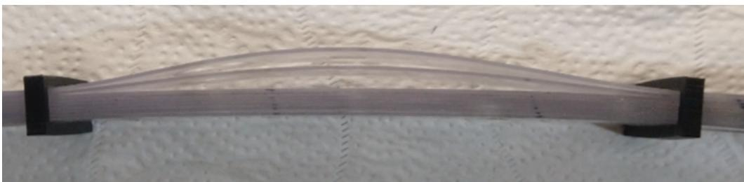
FIGURE 3.5: Buckling of some sheets of the LJS between 2 frames.
