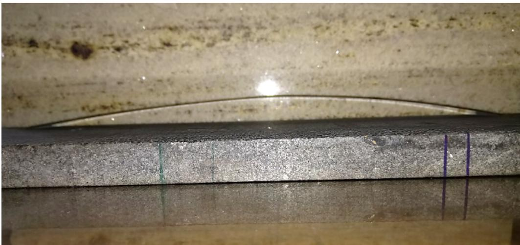
FIGURE 3.9: Deflection of the layers due to the rolling shape of the raw material.
