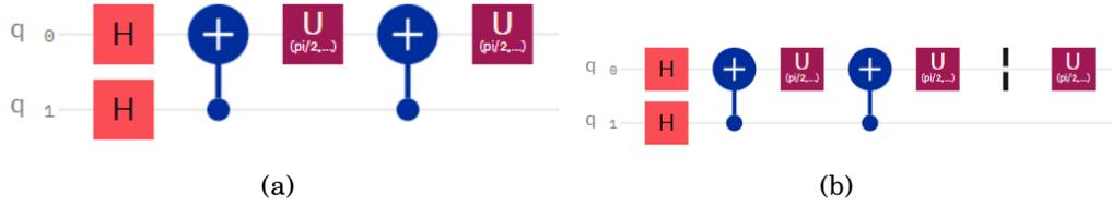
Figure 3.1: (a) Sample circuit showing gate selections for  $H_{\text{cost}}$ . (b) Sample circuit showing gate selections with additional  $U$  gate after barrier for  $H_{\text{mixer}}$ . Note: The sample circuits displayed in the figures represent the building blocks of the actual circuit and do not represent actual angles that are obtained as a solution of VRP using VQE.
