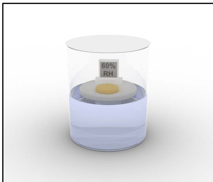
Figure 4.1 Experiment apparatus illustration (inside clear view) for in-door water adsorption experiment. Yellow: hydrogel, grey: polystyrene floating support, blue: DI water.
