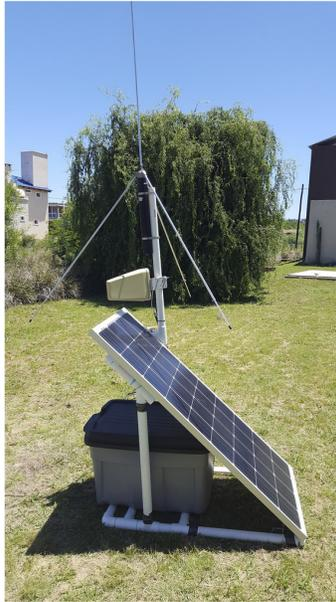
Figure 11. An example of a deployable LMA receiving station that is used along with other LMA stations to map the 4-D structure of lightning within a thunderstorm.
