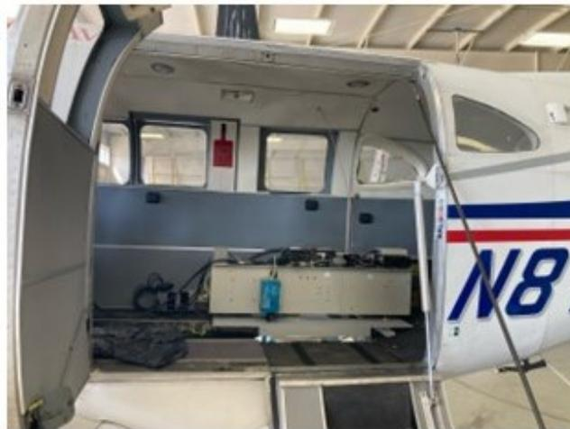
Figure 9. The MCTI camera installed on GLiHT for flights over southern Virginia in July 9-16, 2024.
