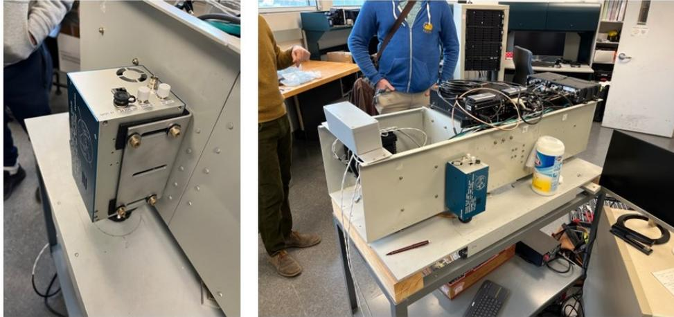
Figure 8. MCTI camera mounted on a Goddard airborne platform (G-LiHT).
