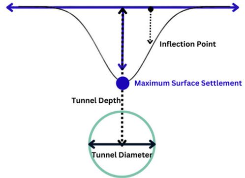
Fig. 3. Settlement perpendicular to the direction of tunnelling.
