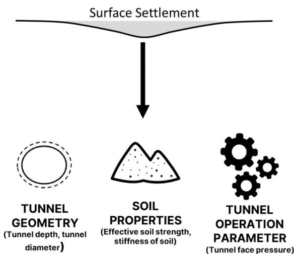
Fig. 8. Three (3) main parameters affect the tunnelling.
