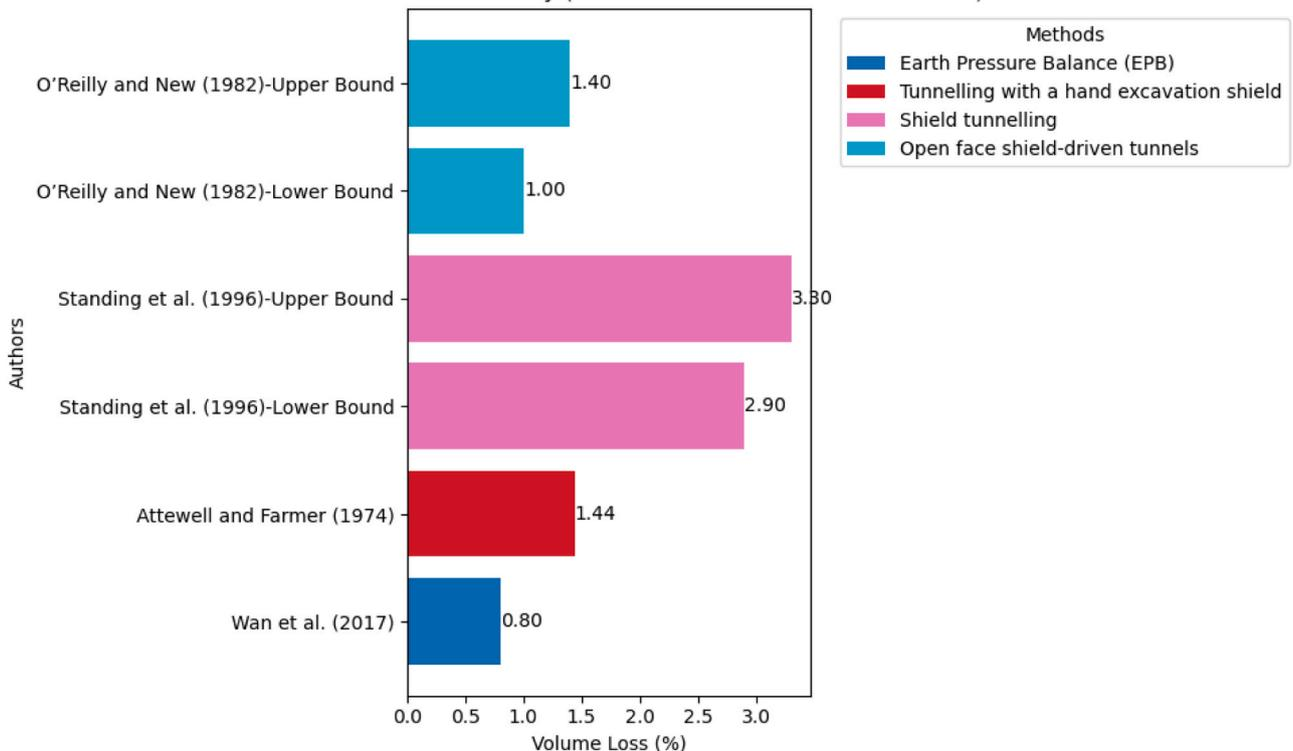
Fig. 5. Volume loss for London Clay with different tunnel excavation.
