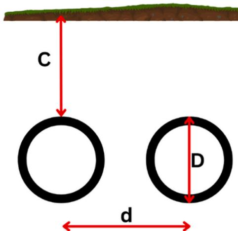
Fig. 11. Geometrical parameters in twin tunnel.
