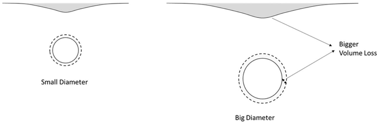
Fig. 9. Illustration of Small and Big Tunnel Diameter impact on the SS.
