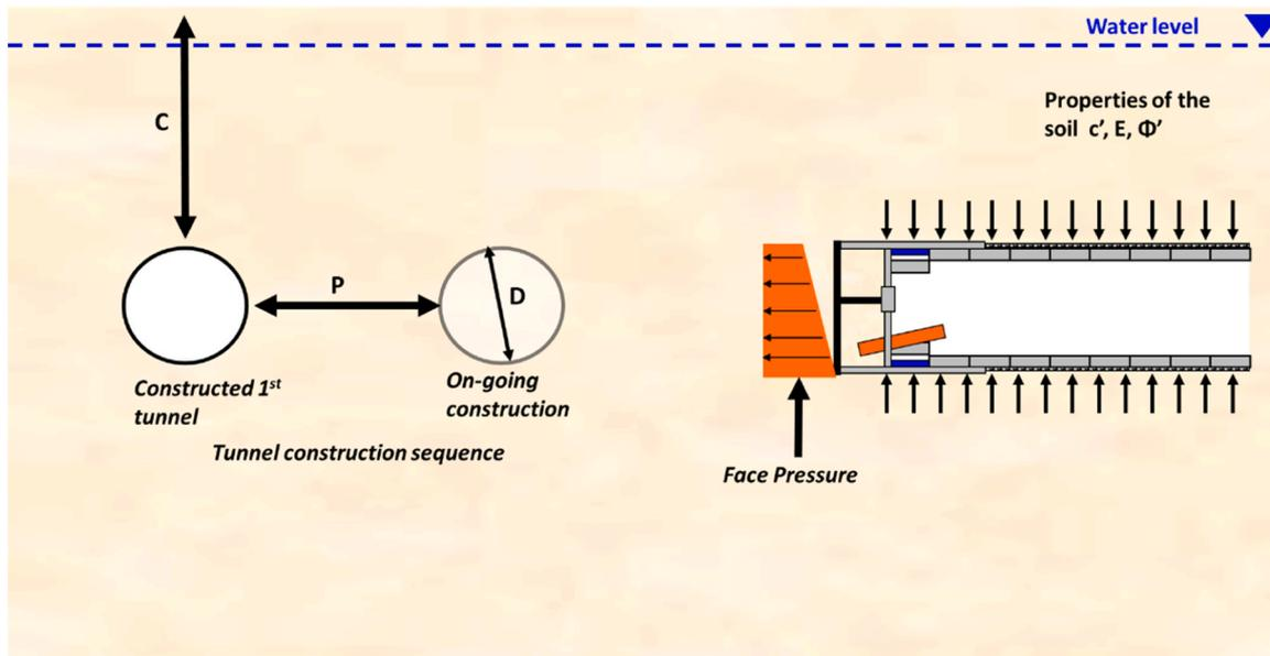
Fig. 12. Summary of the parameters affecting the SS due to twin tunnels.
