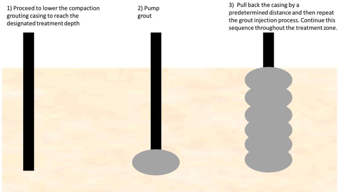
Fig. 14. Simplified process of compaction grouting.
