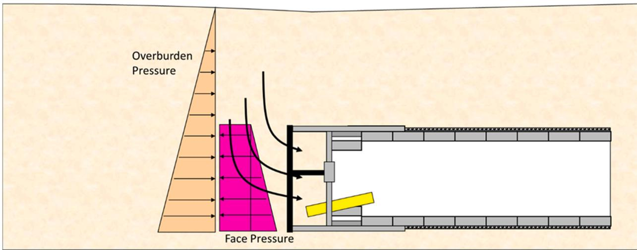
Fig. 7. Face pressure uses to withstand the overburden pressure from the ground.
