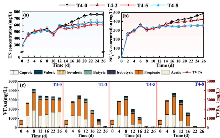
Fig. 3. Effect of biochar on (a) TN, (b)  $\text{NH}_4^+$ -N, and (c) Total volatile fatty acids (TVFA) concentration and fractions of VFAs during anaerobic digestion of food wastewater with 4 g/L oleate-Na.
