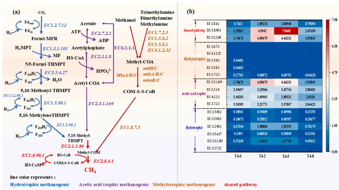
Fig. 6. Effect of biochar on (a) key methanogenic metabolic pathways and (b) the relative abundance of key enzymes in anaerobic digestion of food wastewater with 4 g/L oleate-Na.
