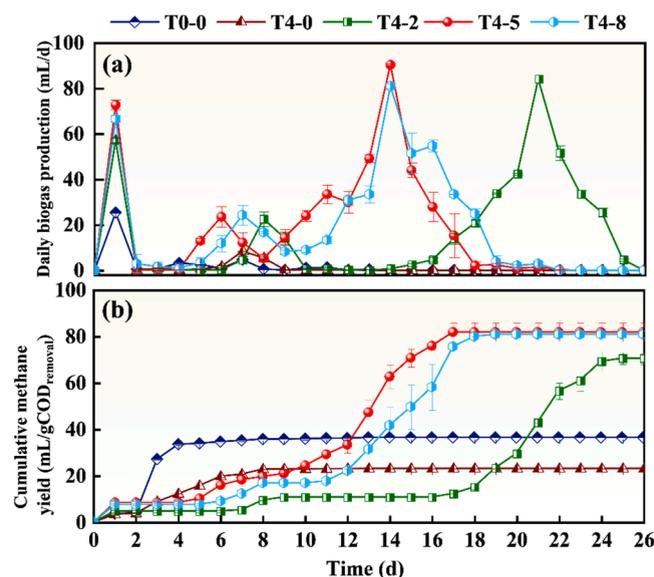
Fig. 1. (a) Daily biogas production and (b) cumulative methane yield under different concentrations of biochar and oleate-Na additions.
