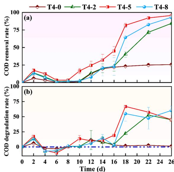
Fig. 2. Effect of biochar on the (a) COD removal rate and (b) degradation rate during anaerobic digestion of food wastewater with 4 g/L oleate-Na.
