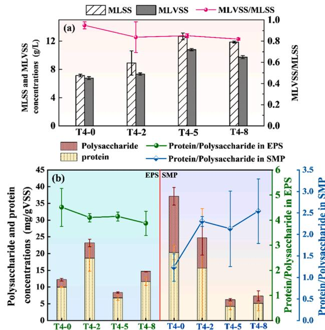
Fig. 4. Effect of biochar on (a) MLSS and MLVSS concentrations and MLVSS/MLSS ratio, and (b) protein and polysaccharide concentrations, as well as protein/polysaccharide ratios in SMP and EPS, during anaerobic digestion of food wastewater with 4 g/L oleate-Na.
