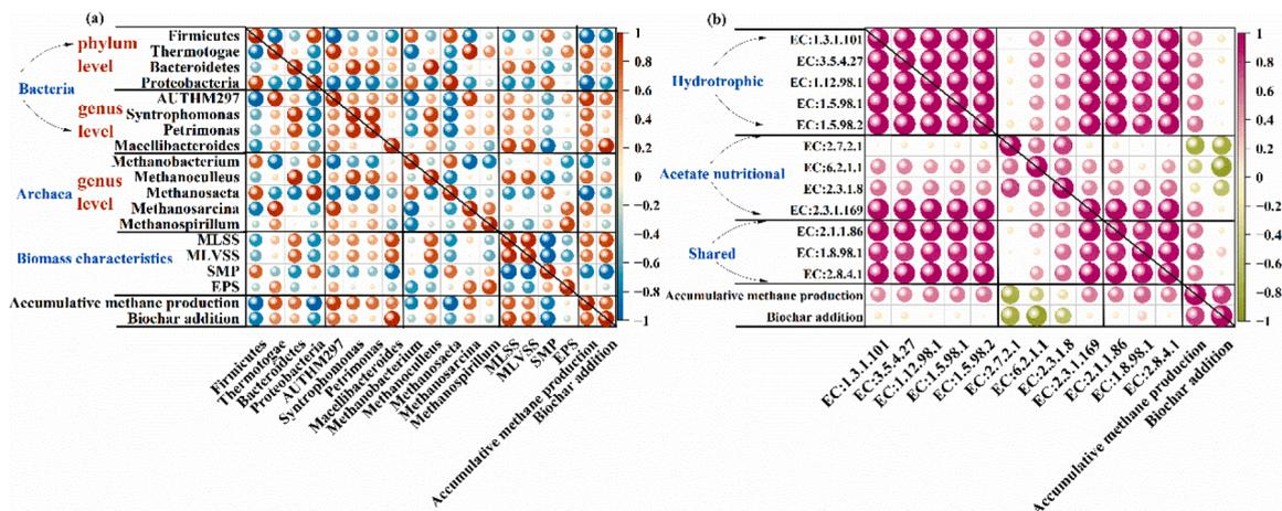
Fig. 7. Correlation analysis of (a) major microorganisms, sludge characteristics and methane production (b) methanogenic key enzymes with methane production in anaerobic digestion of food wastewater with the addition of oleate-Na at 4 g/L.
