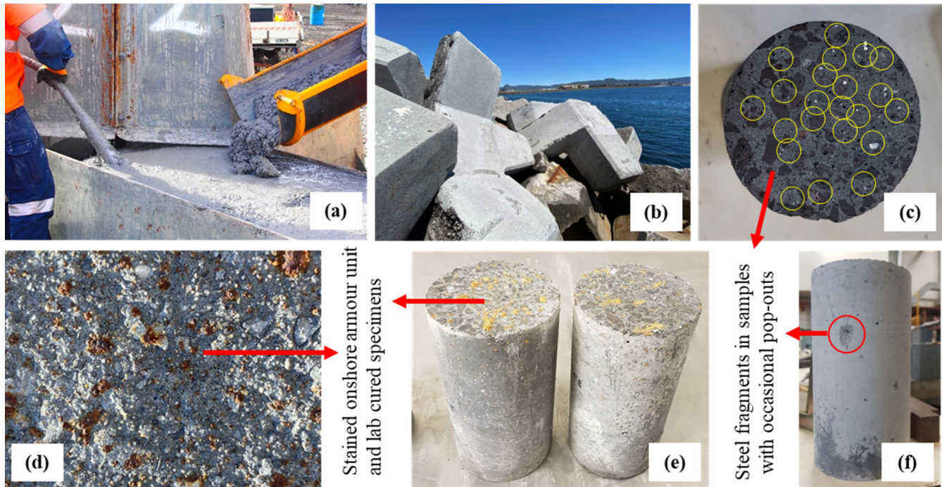
FIGURE 1 (a) Armor unit formwork filling and compaction; (b) GPC Hanbar units within the splash zone; (c) steel fragments visible on specimen surface; (d) stains on the base of a unit; (e) stains on specimens cured in saline water; (f) instance of aggregate popping. GPC, geopolymer concrete.
