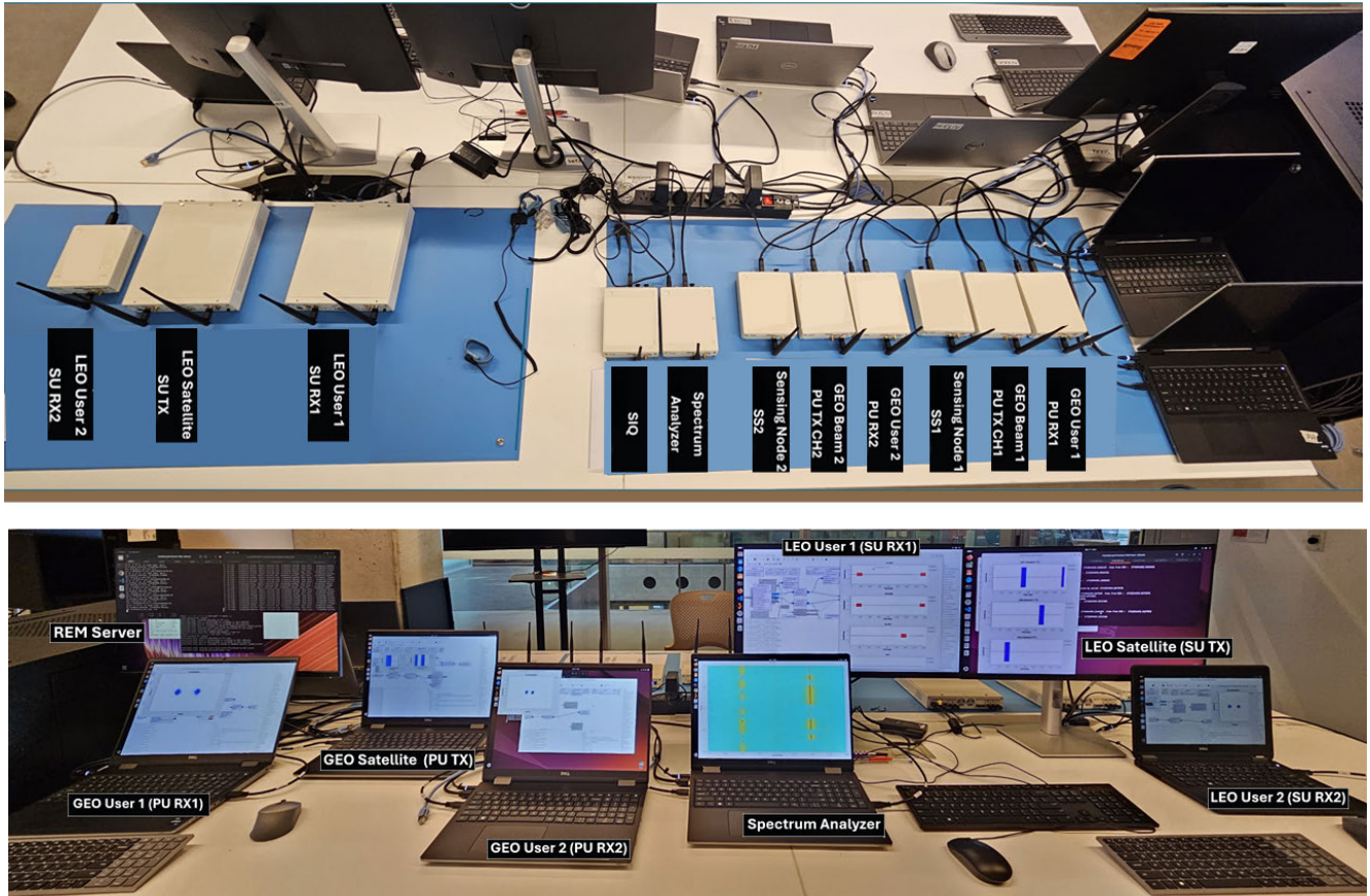
FIGURE 3. The proposed demonstration platform to emulate cognitive GEO-LEO dual satellite system.
