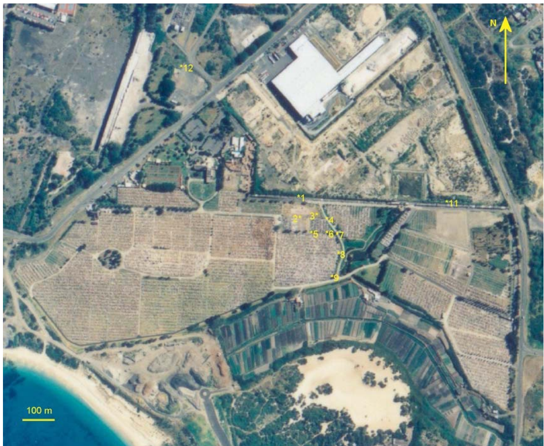
Figure B.2 Piezometer Locations at BOT (aerial photo base – NSW Dept. Lands, 1994)
