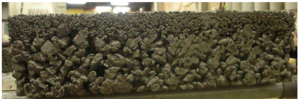
Figure 3.6 Specimen of pervious pavement system
