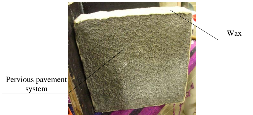
Figure 3.12 Pavement specimens covered by wax
