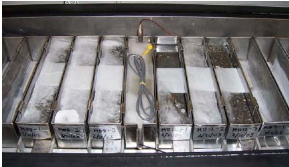
Figure 2.20 Freeze-thaw resistance test for pervious concrete [32]
