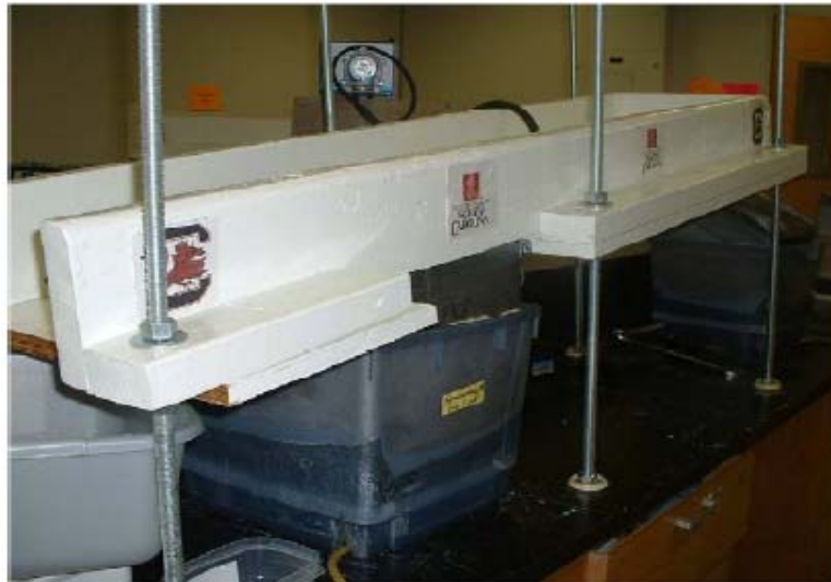
Figure 2.24 Experimental set-up for clogging test [17]
