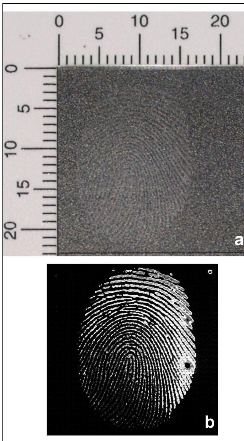
Figure 4.12: Fingerprint (donor #3) treated with 2-cyanoethyl 2-cyanoacrylate on glass slide. (a) White light photograph. (b) Monochrome representation of FTIR chemical image (second derivative, 987\text{ cm}^{-1} ).
