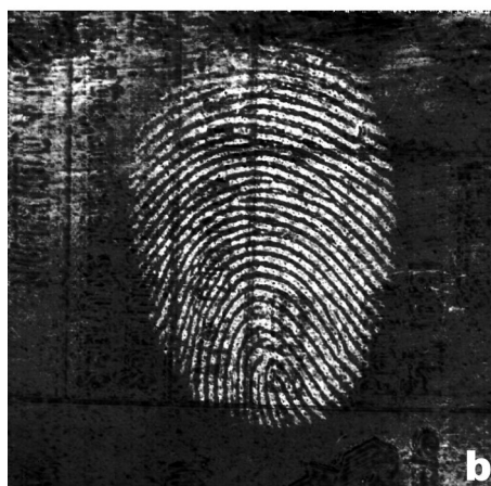
Figure 2.9: Ethyl cyanoacrylate fumed fingerprint on Lift aluminium drink can. (a) White light photograph. (b) Monochrome representation of FTIR chemical image.
