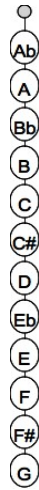
Figure 4.3: The mass-spring model for Partial Reflections I . Circles represent masses and connecting lines represent springs. The smaller, shaded sphere's position is fixed, all others are mobile masses.
