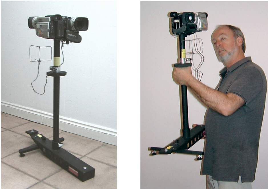
Fig. 5.18: Two-camera handheld mount, with wireframe viewfinder.
