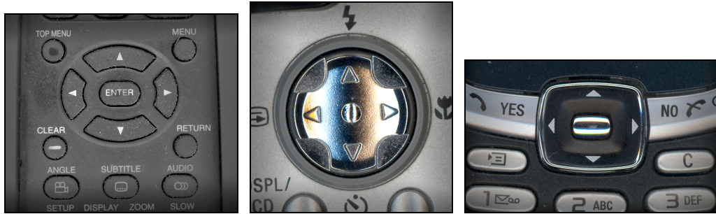
Fig. 5.37: 4/5-way navigator, l-r: DVD controller; digital camera; mobile phone
