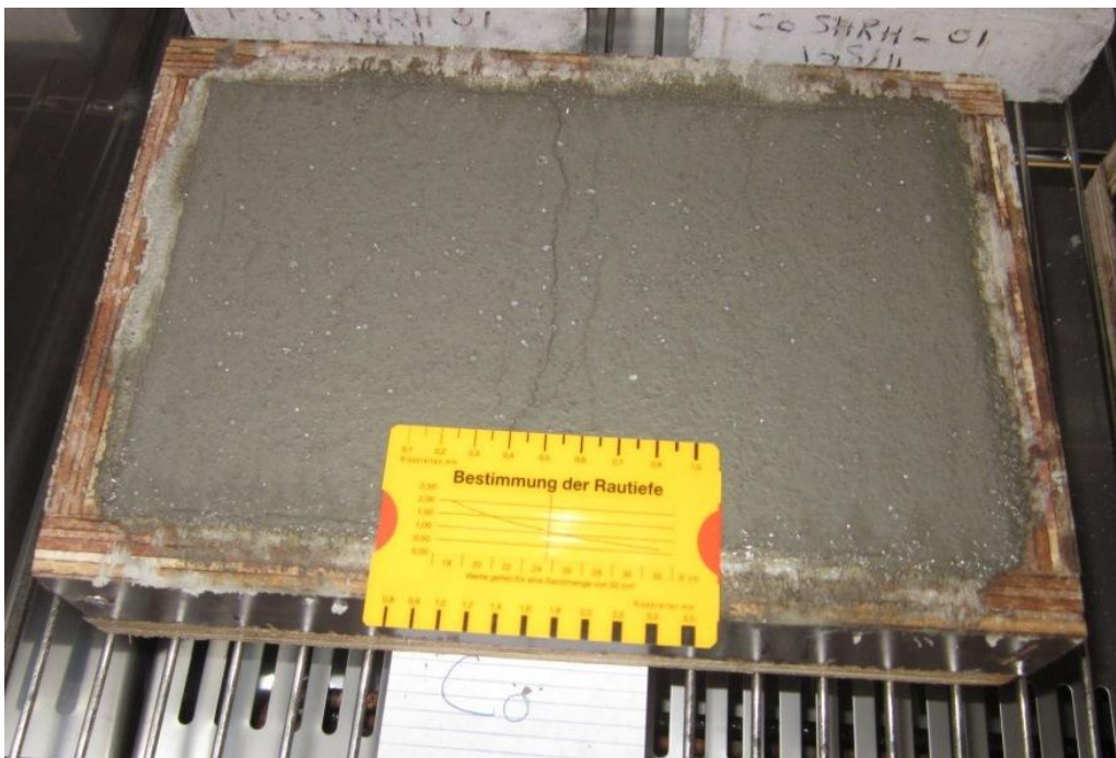
Figure A. 7. Early age cracking of control sample after 24 hours
