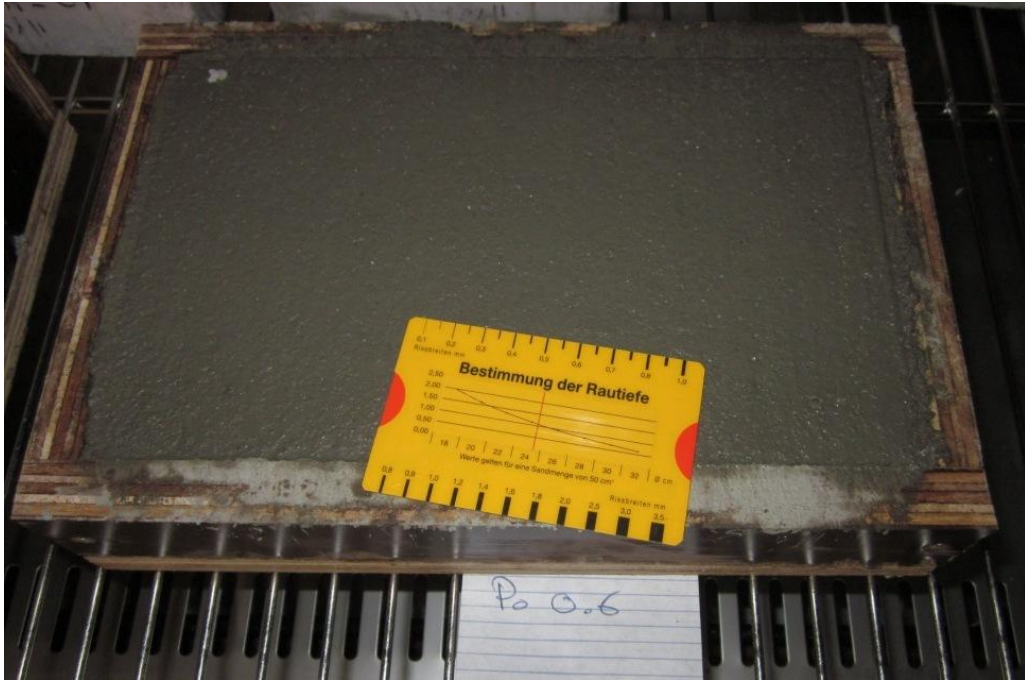
Figure A. 8. Early age cracking of APP0.6 sample after 24 hours
