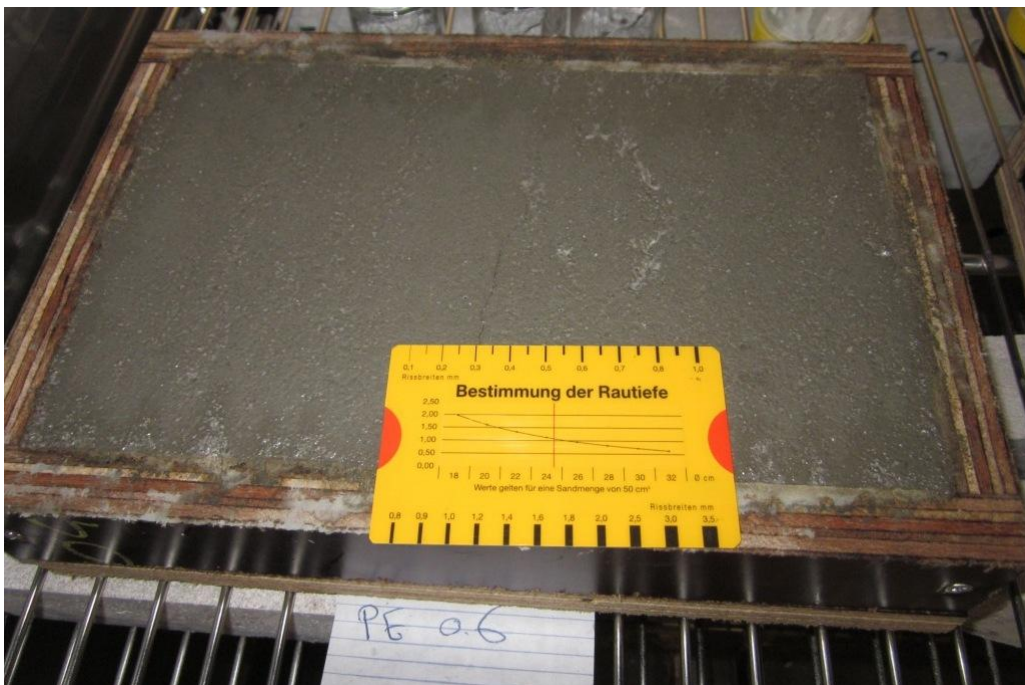
Figure A. 9. Early age cracking of PE0.6 sample after 24 hours
