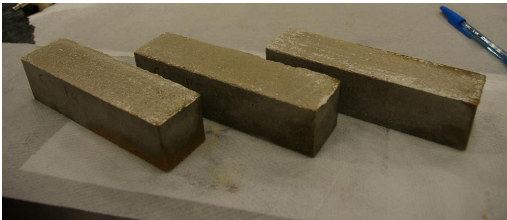
Figure A. 5. After exposure to sulphate solution (control specimens)
