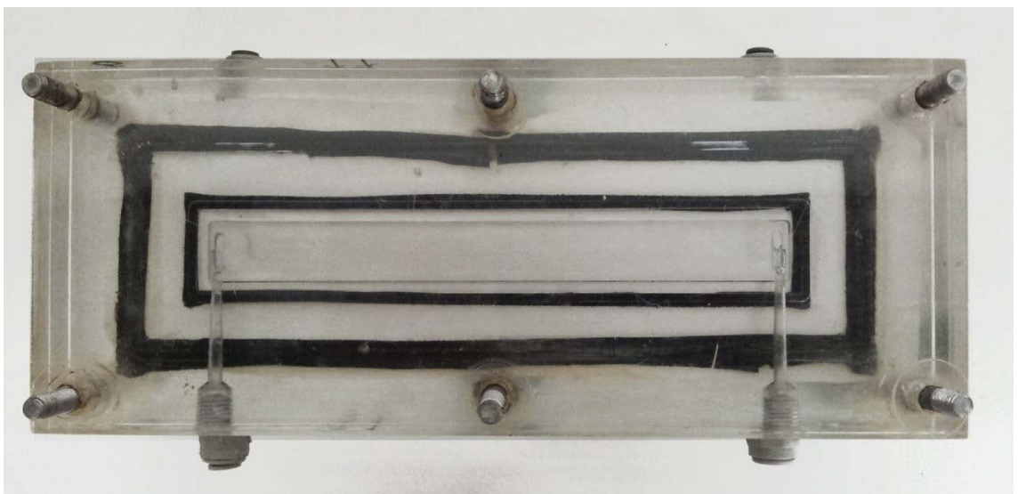
Fig. 3.6 Overhead view of FO test cell with active flow cell of 2 x 21 x 0.3 cm on each side of the cell and double sealing
