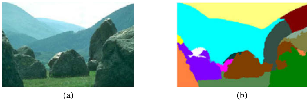
Figure 5.1: An example of image segmentation. (a) The original image. (b) The segmentation result of (a). Sub-regions are represented by different colours (courtesy Zhang [8]).
