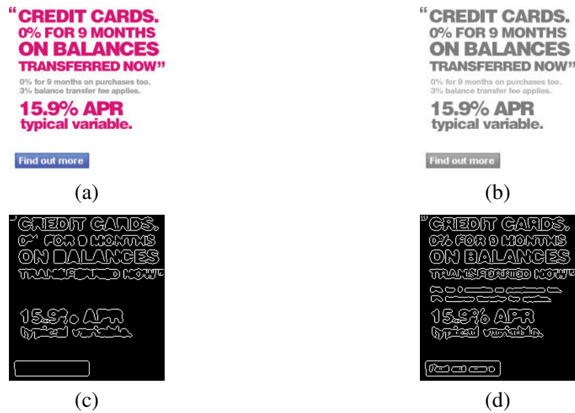
Figure 3.3: An example of Canny edge maps obtained with different thresholds. (a) The original colour image. (b) The gray-level image of (a). (c) The Canny edge map of (b) with high thresholds. (d) The Canny edge map of (b) with low thresholds.
