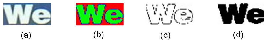
Figure 5.11: A comparison between the binarisation results obtained using M metric in [9] and that using the proposed M_{norm} metric with Euclidean Distance. (a) Original image. (b) 3-means clustering result with Euclidean Distance. Here, the green, red and blue colours represent the textual foreground cluster, background cluster and the noise cluster respectively. (c) Binarised text (in black) by using M . (d) Binarised text (in black) by using M_{norm} . (Best viewed in colour).
