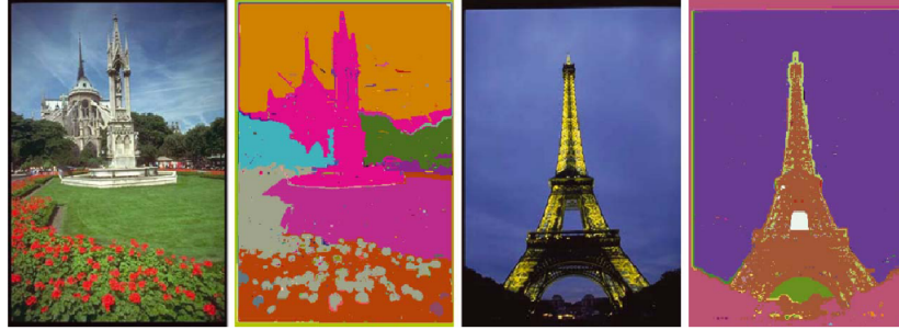
Figure 2.6: Results of minimum spanning tree-based image segmentation (courtesy of [6]).
