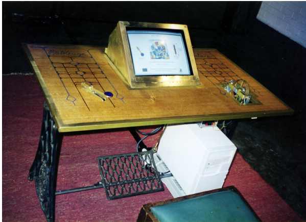
Figure 4. Stephen Jones' Reading Machine . Note Morse key to left and navigation wheel to right of monitor. © Stephen Jones
