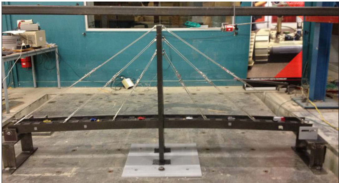
(a) Bridge model on the shake table
