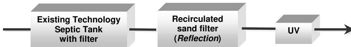
Figure 11: Concept diagram of the technologies in Option 2 .
