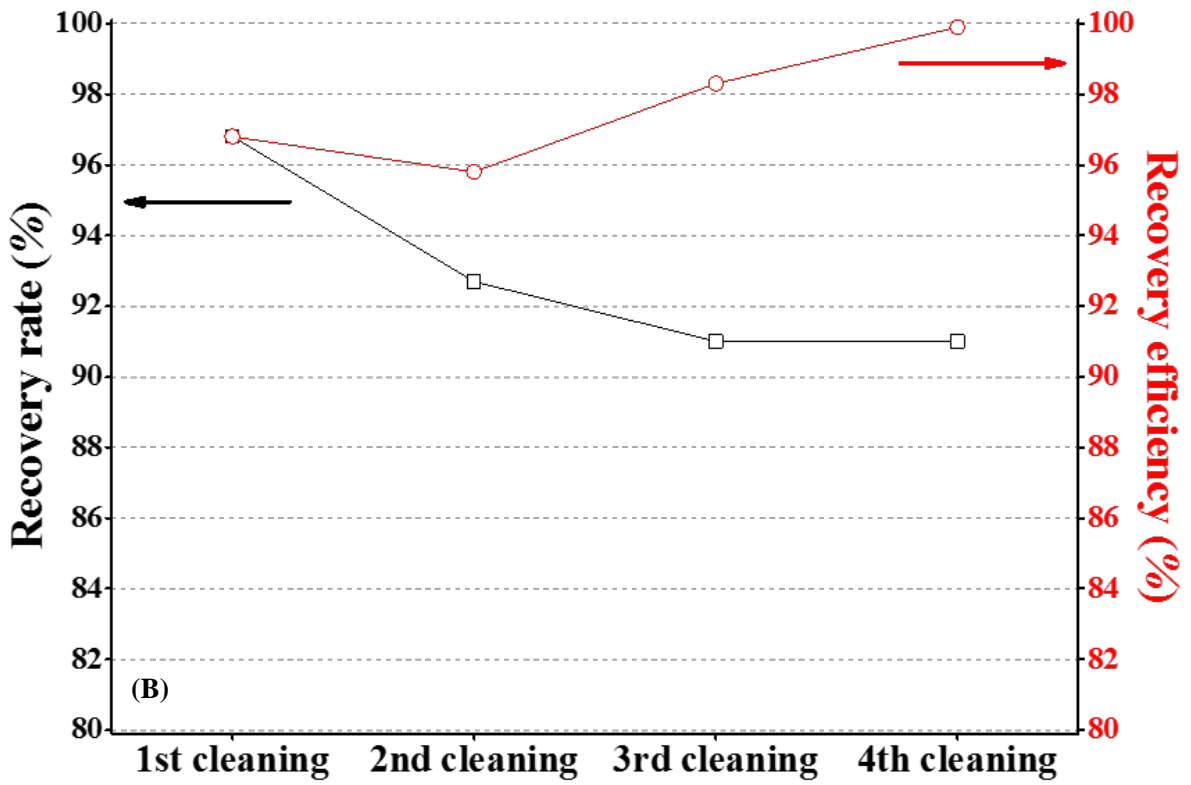
Figure 5. (A) Flux and (B) recovery rate and efficiency using chemical cleaning process
