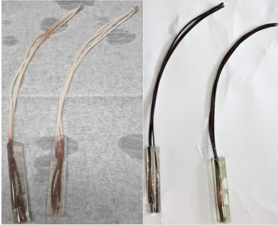
Figure 2. Hollow fiber membrane before and after chemical cleaning ( \text{pH} \geq 12 )
