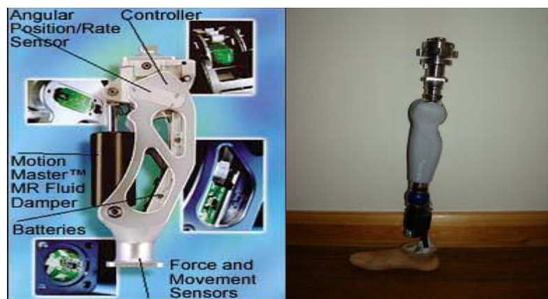
Figure 2.37. MR damper applied in lower leg prosthesis
