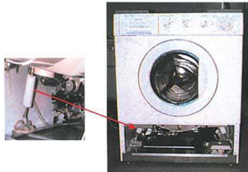
Figure 2.36. MR damper installed in a washing machine
