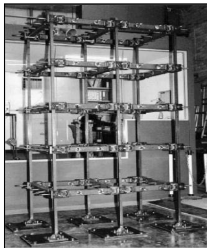
Figure 6.26. Five storey benchmark steel frame
