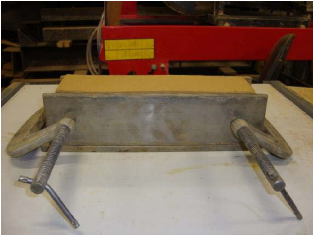
Figure 4.4 Preparation for removing uneven part on top surface of mortar prism
