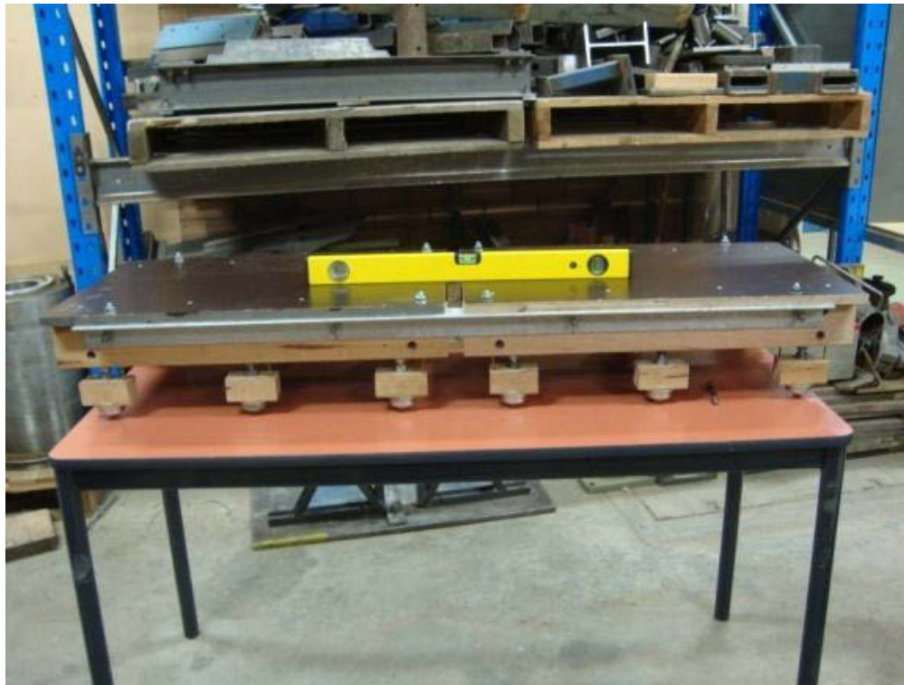
Figure 5.15 A base for supporting wall specimen for bending test in lateral span
