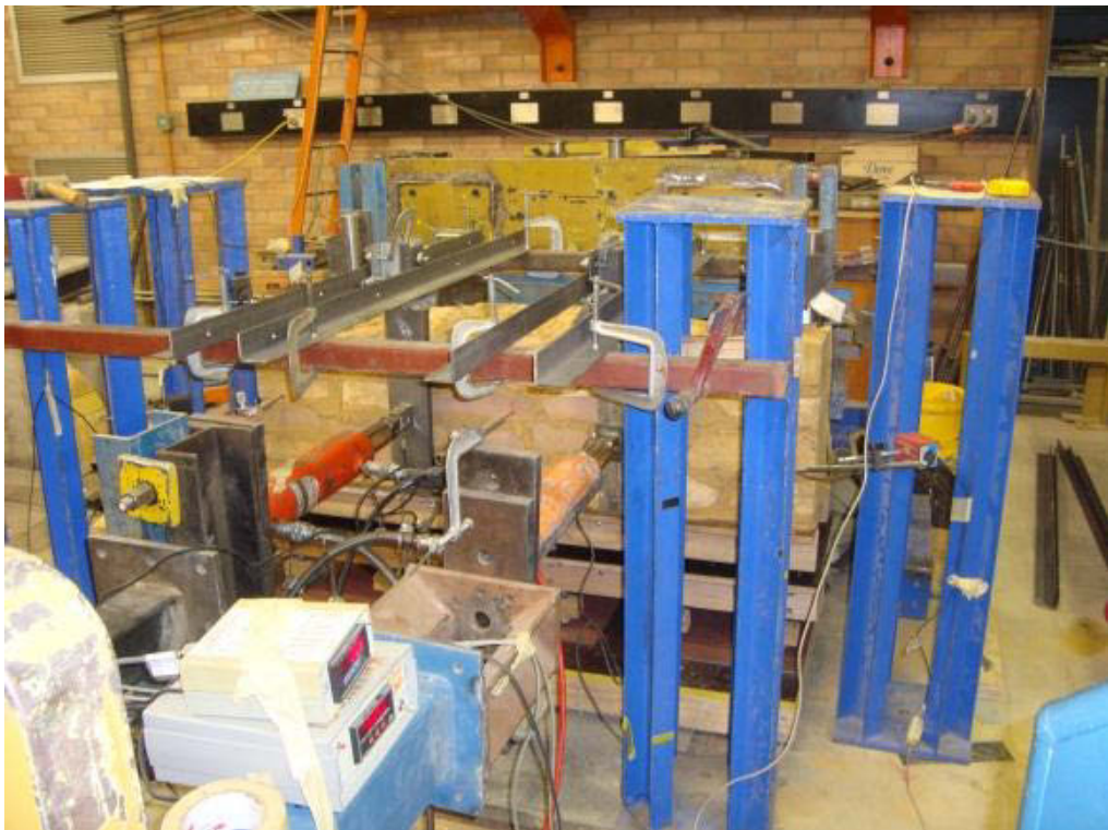
Figure 5.41 Bending test of a wall specimen in lateral span
