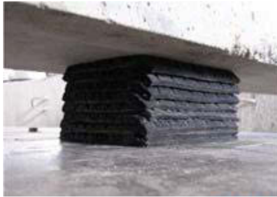
Figure 2.19 Scraped tyre pads used as a base isolator (Turer & Özden 2008)
