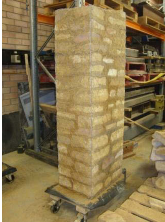
Figure 5.13 Reinforced wall specimen using prefabricated mesh
