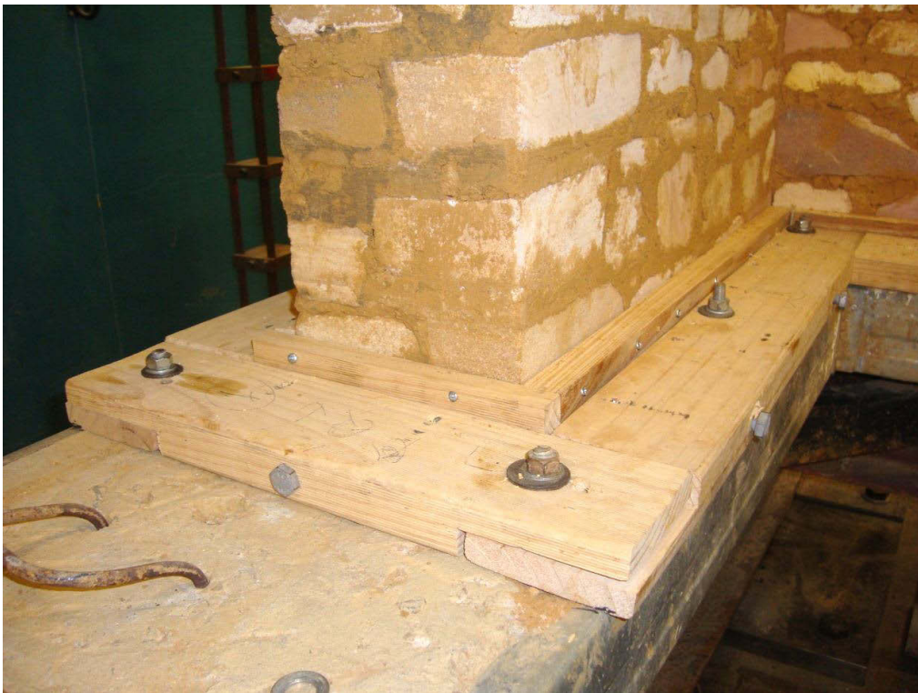
Figure 5.24 Additional anchorage provided to the specimen
