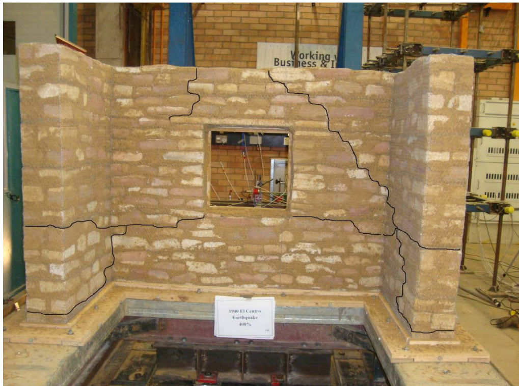
Figure 5.62 Cracks in the main wall after 400% loading intensity
