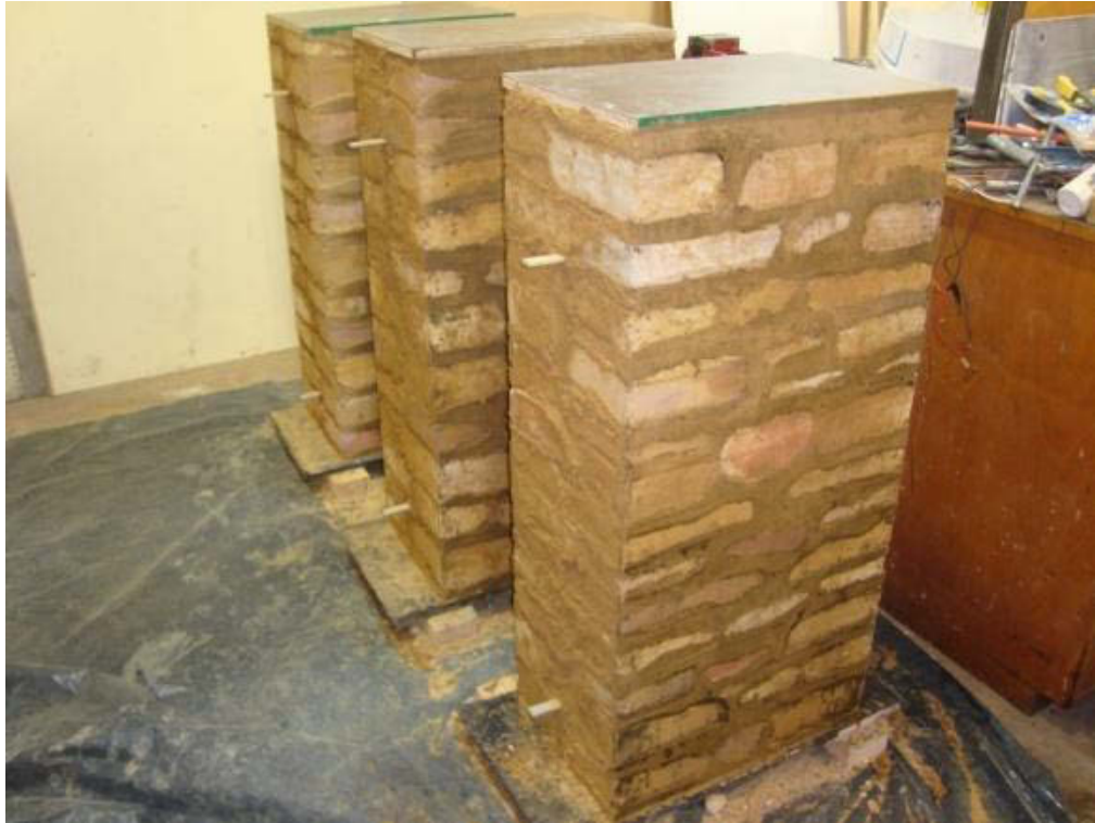
Figure 5.2 Wall specimens for compression test
