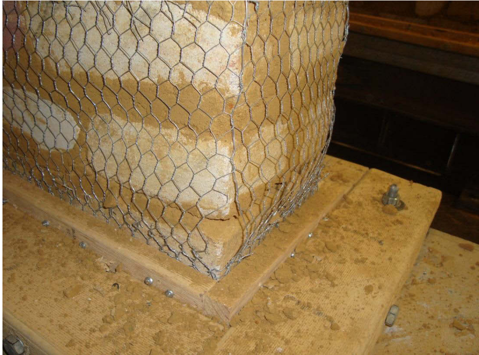
Figure 5.58 Joint unwoven at 375% loading intensity
