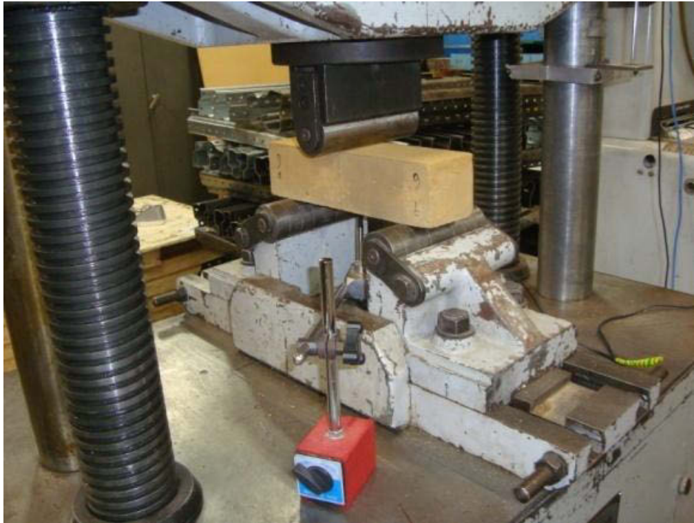
Figure 4.14 Mud mortar beam under flexure test
