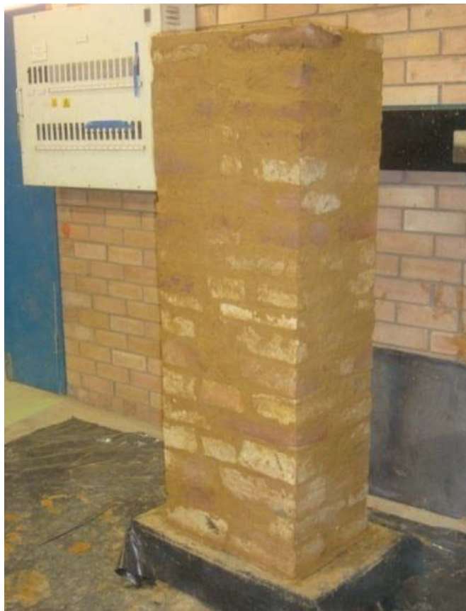
Figure 5.4 Specimen for flexure test in vertical span
