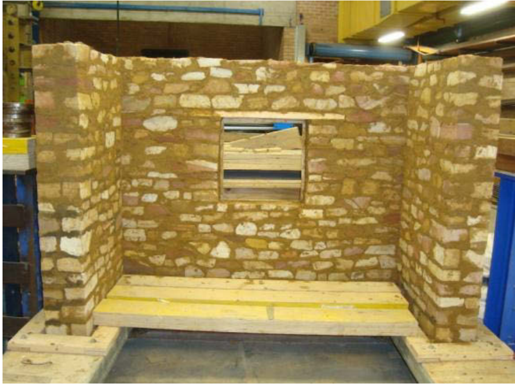
Figure 5.22 Un-reinforced specimen for shake table testing
