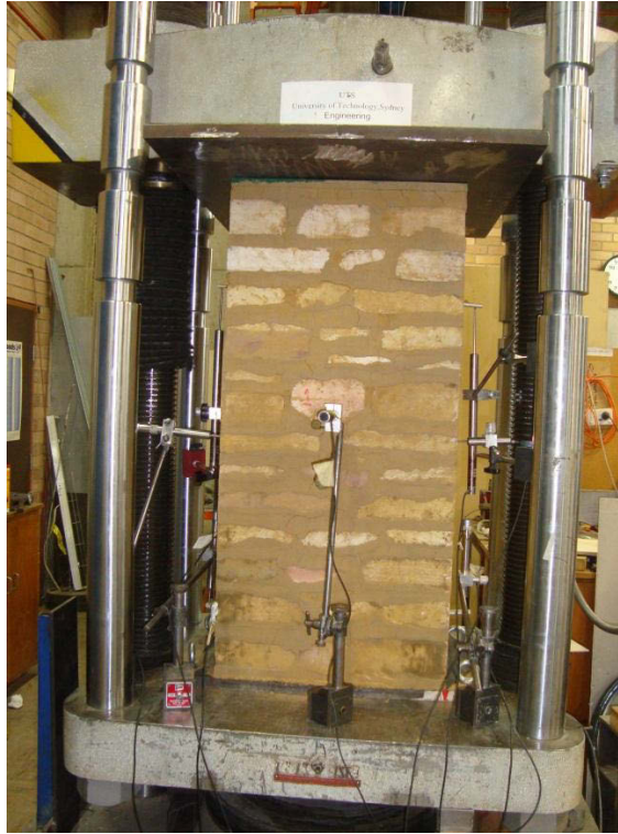
Figure 5.31 Wall specimen during compression testing
