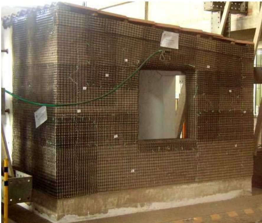
Figure 2.17 Geo-mesh reinforcement (Blondet, Vargas & Rubiños 2009)
