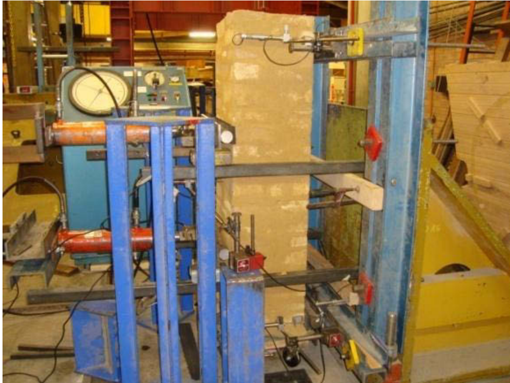
Figure 5.35 Wall specimen under bending test in vertical span
