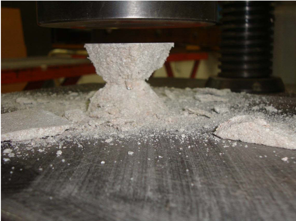
Figure 4.19 Specimen after failure
