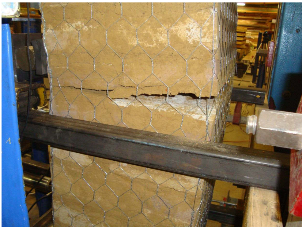
Figure 5.38 Crack in reinforced wall specimen (Bending in vertical span)
