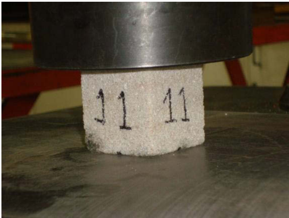
Figure 4.18 Stone cube under compression test
