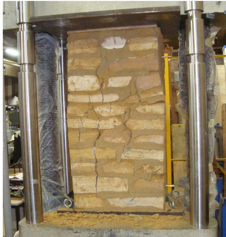
Figure 5.33 Wall specimen on the verge of collapse
