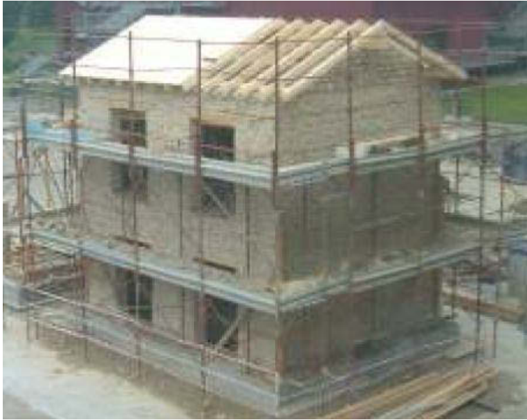
Figure 2.36 Specimen before fixing clay tiles (Magenes, Penna & Galasco 2010)
