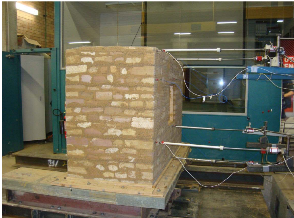
Figure 5.54 Reinforced wall specimen during testing
