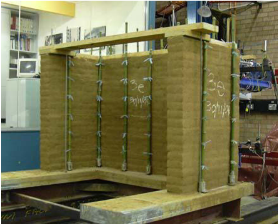
Figure 2.18 External bamboo reinforcement (Dowling, Samali & Li 2005)
