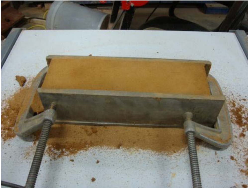
Figure 4.5 Mud mortar prism with a smooth top surface
