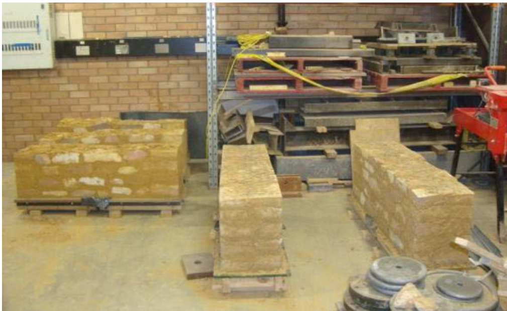
Figure 5.18 Wall specimens for bending test in lateral span.
