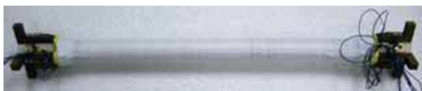
Figure 2 A 1.6 kA experimental DC cable made using 2G HTS wires
