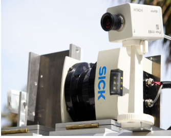
Fig. 7. The camera and vertically mounted laser.
