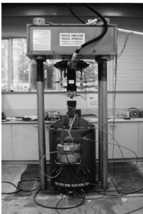
Fig. 4. Cylindrical triaxial apparatus with dynamic actuator designed at University of Wollongong
