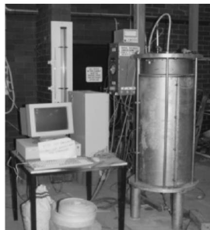
Fig. 9. Large-scale consolidometer built at University of Wollongong (Indraratna and Redana, 2000)
